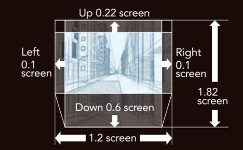
\* This figure shows the lens shift range for the projector with the optional lens SD-903 at the ceiling mounting position.
